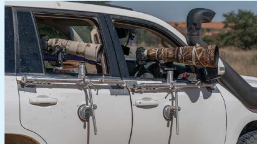
Close-up of the commercially available door mounted camera support systems attached to the Landcruiser (Etosha, Namibia)
