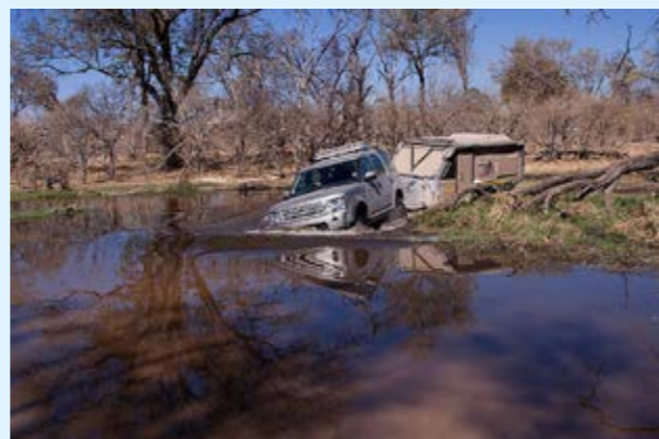
Crossing a river when towing a caravan can be dangerous if you get stuck in the mud. You must therefore be very sure that you will be able to get through by walking the planned path through the water first
