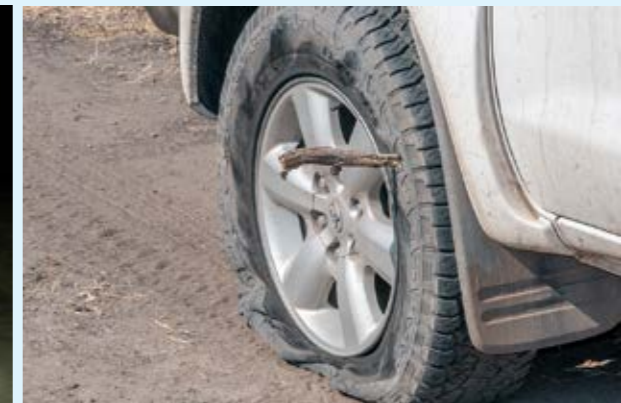
Deflating the tyres to a third or more of the normal pressure is a huge assistance for sand driving but makes the tyre side walls much more prone to punctures (Namibia)
