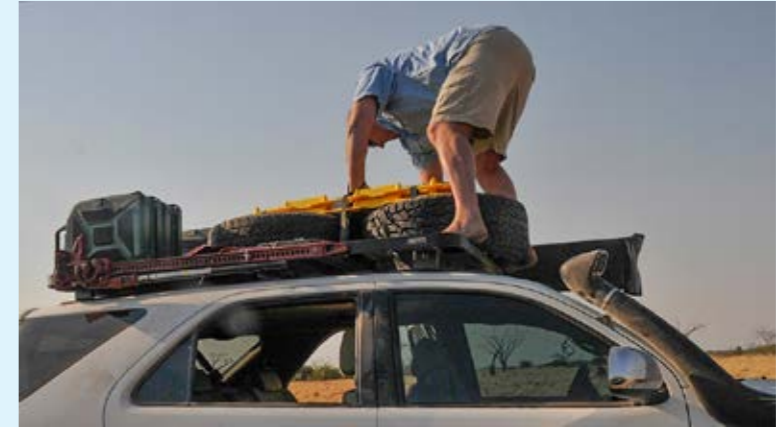
The roof rack is essential, but should not be overloaded as it will make the vehicle top heavy
