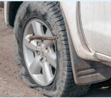
Deflating the tyres to a third or more of the normal pressure is a huge assistance for sand driving but makes the tyre side walls much more prone to punctures (Namibia)
